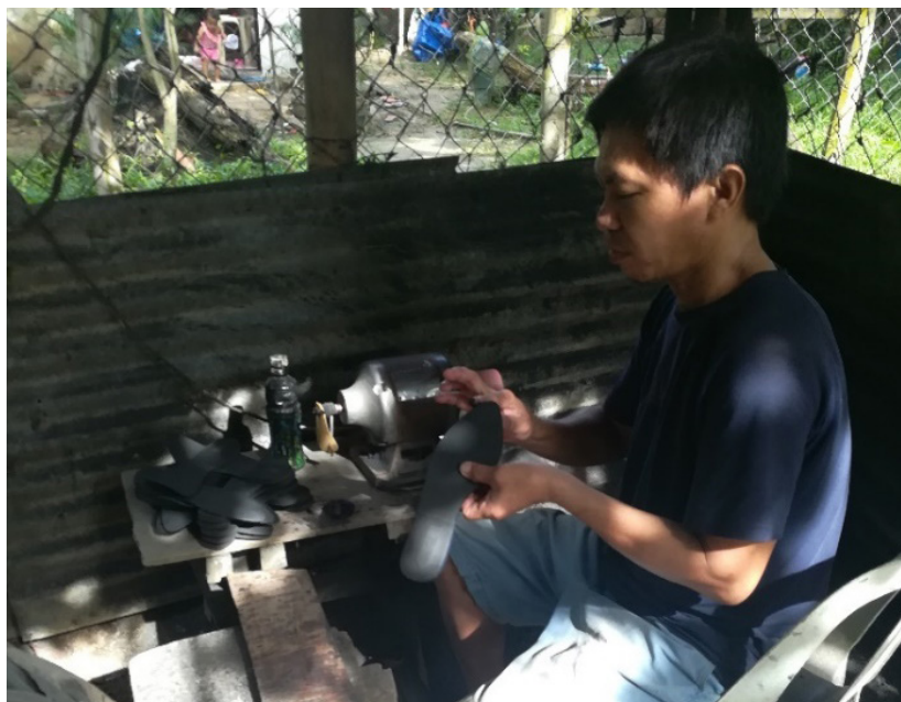
Figure 9. Preparing the outer sole to be smoothed using the grinder (found on the right side of the shoemaker)
