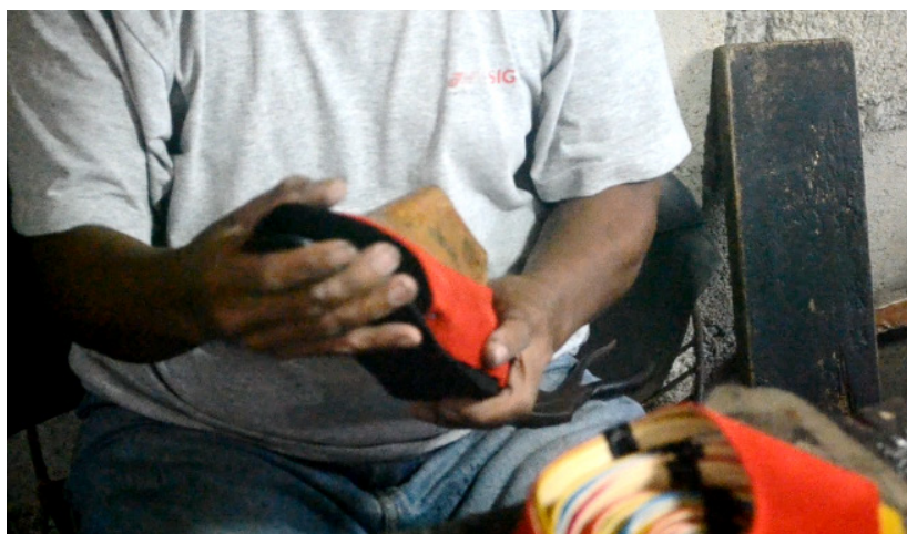
Figure 10. Fitting the upper part of the shoe to the shoe last
