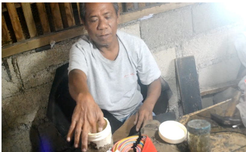
Figure 7. Putting adhesive on the sole-shaped cardboard before attaching the rubber (for the insole)
