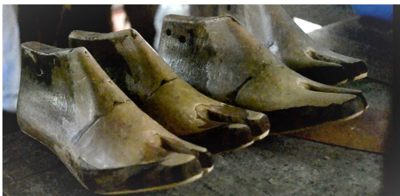
Figure 11. Wooden shoe lasts that have been repaired for the new types of shoes being made
