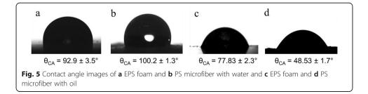
gas interface under the water droplet that may improve PS microfibers' hydrophobicity compared to untreated EPS foam [27]. Meanwhile, a contact angle of 48.5 ± 1.7° was observed for the PS microfibers with mineral machine oil as the test. This is notably smaller than EPS foam's oil contact angle value ( $\theta_{CA} = 77.8 \pm 2.3^\circ$ ), signifying the PS microfibers' improved oleophilic behavior.
