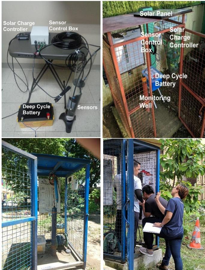
Figure 5: Test setup in a controlled environment (top-left), the setup installed on some of the groundwater monitoring wells (top-right, bottom-left), and the team during one of the system installations (bottom-right)
