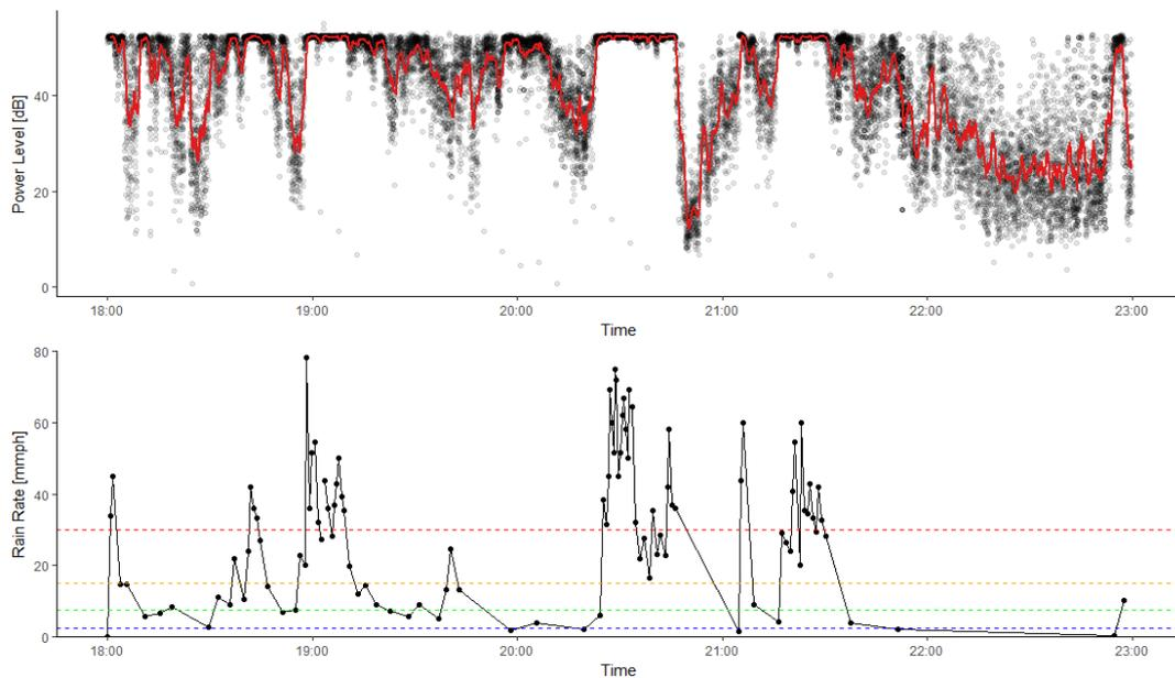
**Figure 5.** Sample rain rate and acoustic power level visualization for a 5-hour rain event in Infanta, Quezon weather observation site last November 24, 2017
