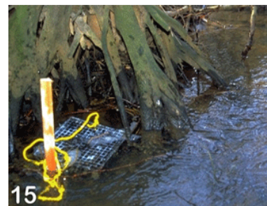
Figures 15: A colonization basket filled with natural substrates and exposed in a river.
