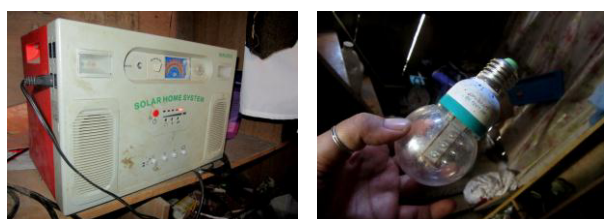
Figure 6. The SHS charge controller with radio feature, and the 12V, 1.2 W LED bulb that came with the SHS.
