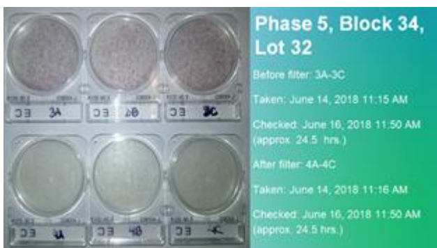
Figure 2: Water test kits showing results of contaminated (above) and cleaned water (below) in one installation site
