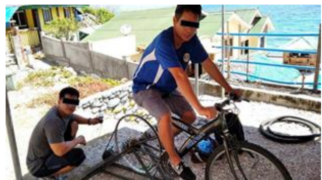
Figure 4: Pedal-powered alternator installed at Isla Verde, Batangas
